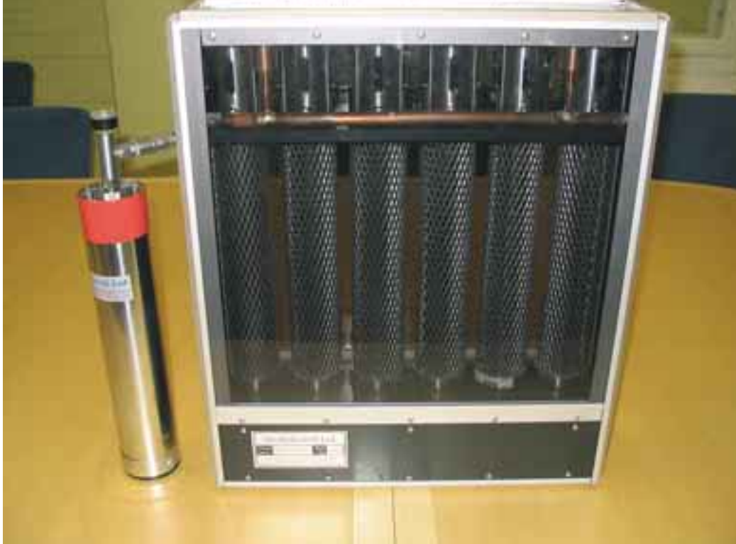
HC600 fuel cell accumulator (10A, 14.5V) equipped with a regenerable carbon dioxide filter.
