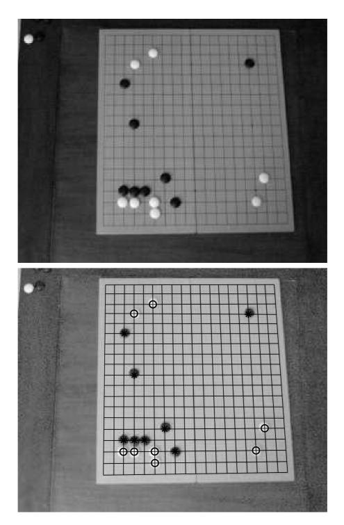
Figure 7: Test image 1 ( $320 \times 240$ ): Top: The original image. Bottom: The analysis of the system. Black stones are marked with asterisks, white stones with circles.
