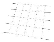
Figure 6: When grid is grown, the lines are extrapolated in opposite directions (solid lines). The goodness of a direction is evaluated by looking how well the extrapolated segments fit to the line image  $I_L$ .
