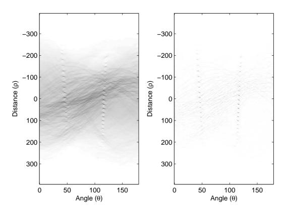
Figure 4: Left: Hough transform  $I_H$  computed from the line image  $I_L$ . The parallel grid lines of the original image form vertical series of peaks in the Hough space. Right: Filtered version of the hough transform of the enhanced line image  $I'_L$ .
