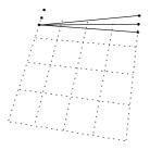
Figure 5: Optimising the position and angle of the topmost horizontal line. Each line is optimised separately by considering a few end points along the perpendicular border lines.
