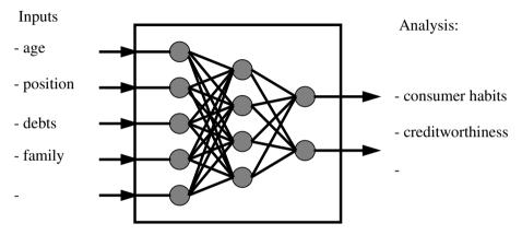
**Principle of neural modeling.** The inputs are known or they can be measured. The behavior of outputs is investigated when input varies.
