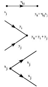
Example: Signal flow graph of linear combination
