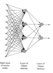
Fully connected 10-4-2 feedforward network with 10 source (input) nodes, 4 hidden neurons, and 2 output neurons.
