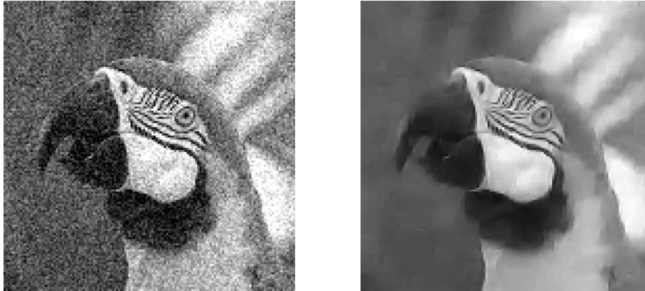
Figure 51: Image denoising by sparse code shrinkage. Using the theory of noisy ICA, one we have developed an image denoising method. This leads to a thresholding of the coefficients of the wavelet-like features shown in Figure 2.
