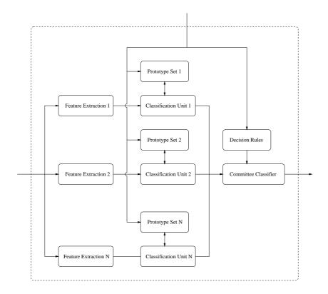
Figure 2: Architecture of the recognizer unit.
