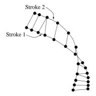
Figure 4: Optimal matching of data points found by the DTW algorithm.
