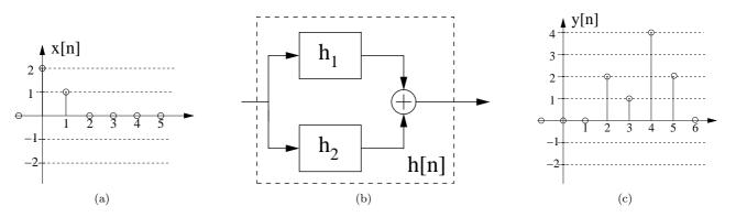
Figure 1: Figures for Problem 2: (a) Input x[n], x[n] = 0, when n < 0, n > 1, (b) LTI-system, (c) Output y[n], y[n] = 0, when  $n < 2, n > 5, n \in \mathbb{Z}$ .
