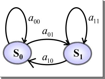
"Observable Markov Model" : output of the process is a set of states.
