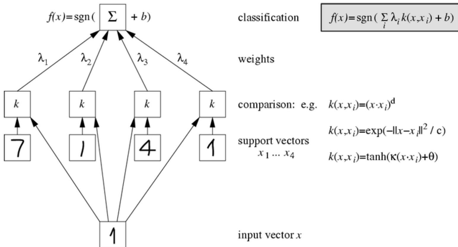
Kuva 4: SVC as a neural network. Each neuron in the hidden layer computes the kernel function between the input pattern '1' and some support vector  $x_i$  for which  $\lambda_i = y_i \alpha_i \neq 0$ .
