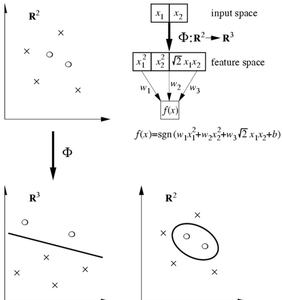
Kuva 3: This is an example on how a nonlinear SVC works.
