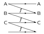
$P(y = A | x = A) = 1 - f \quad P(y = B | x = A) = f$   $P(y = B | x = B) = 1 - f \quad P(y = C | x = B) = f$ ...
