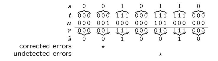
Repetition Codes - Block Codes - Channel capacity
