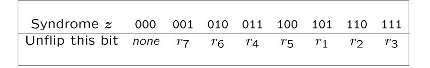
Repetition Codes - Block Codes - Channel capacity
