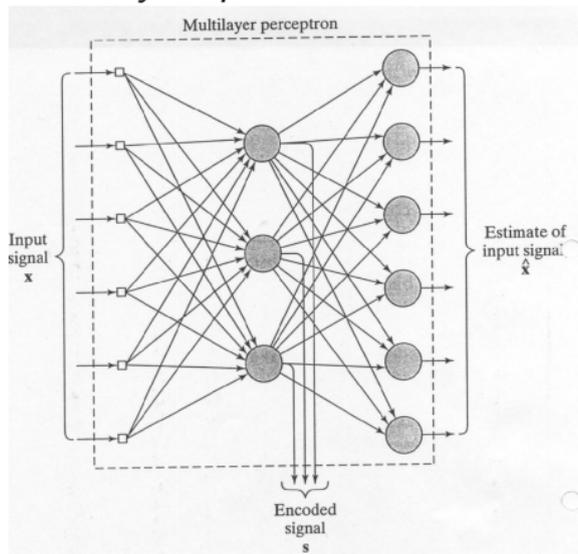
Replicator network with a single hidden layer used as an encoder.
