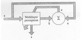
• Block diagram for the supervised training of the replicator network
