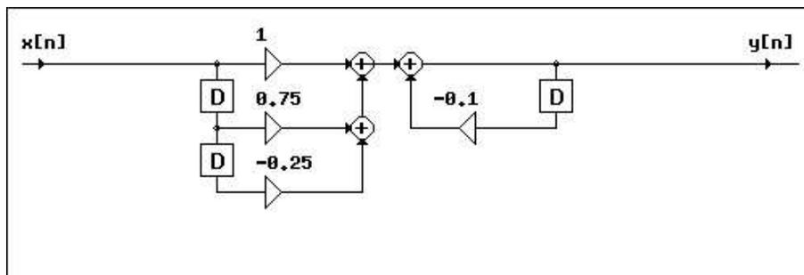
Figure 1: Filter of Problem 2. All memory registers are initially zero.
